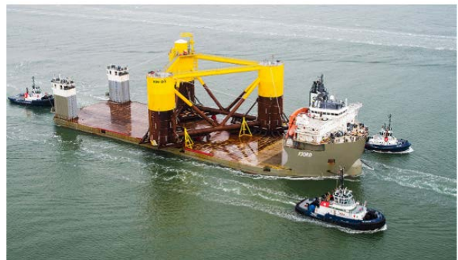
Figure 8 Substructure dry transport (courtesy Boskalis)
