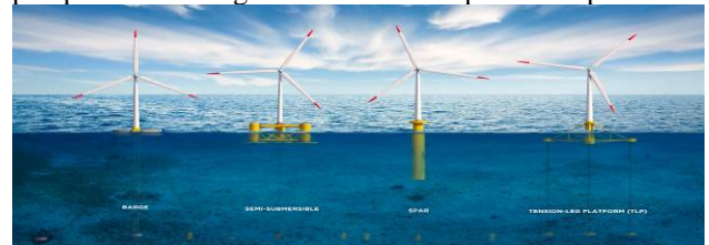
Figure 1 Floating options (courtesy ciervoenergy)
